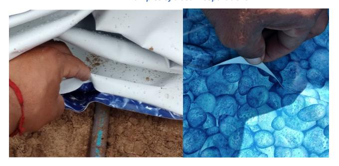
Sometimes liners can develop holes that are not in the seam. These holes can easily be patched even under water. Examples of holes that are not covered by warranty and would need to be patched by customer:
